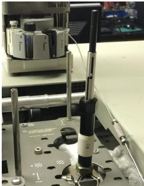
Figure 2.6 SPME inserted into the injection port of the GC-MS
