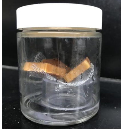
Figure 2.3 VOC experimental setup showing aluminum mesh positioned on the polycarbonate tube ring supporting three wood replicates above sterile water
