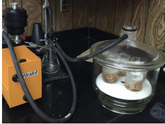
Figure 2.7 Water treatment of wood samples under vacuum before crushing tests
